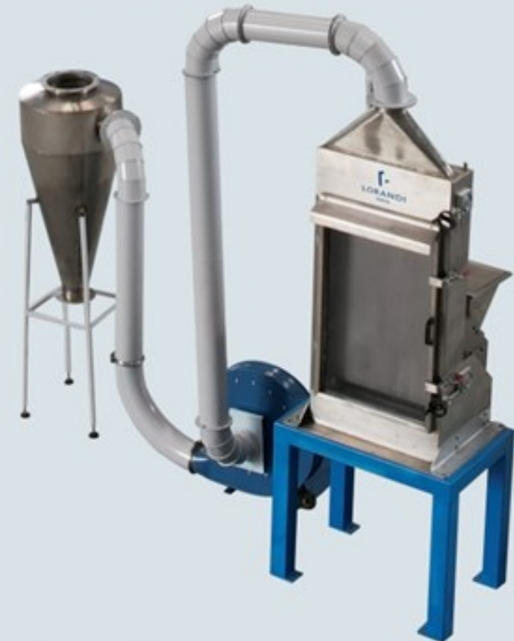
Separation based on bulk density
