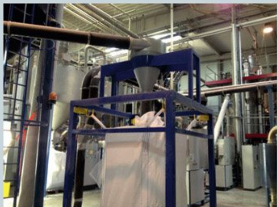
Big-bags discharge station for flakes, PET, PE, Film, PS scraps complete with discharge ampoule
