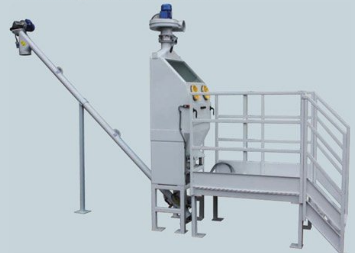
Manual bag breaker Manual bag opener with vibrating cone and screw
