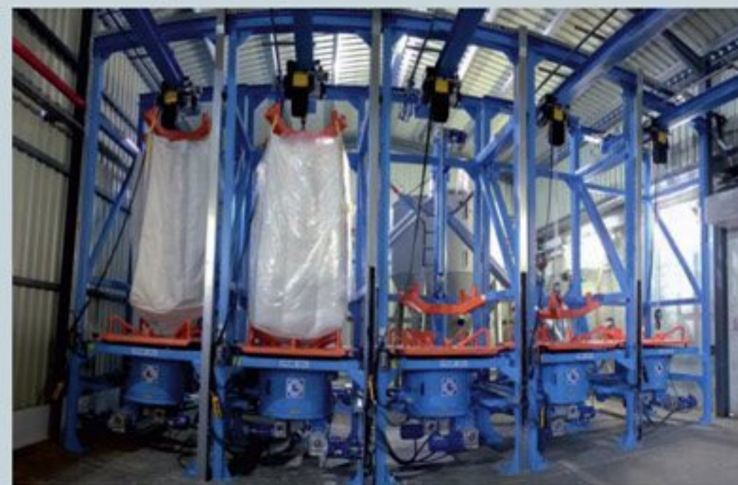
Big-bags discharge station for flakes, PET, PE, Film, PS scraps complete with discharge ampoule
